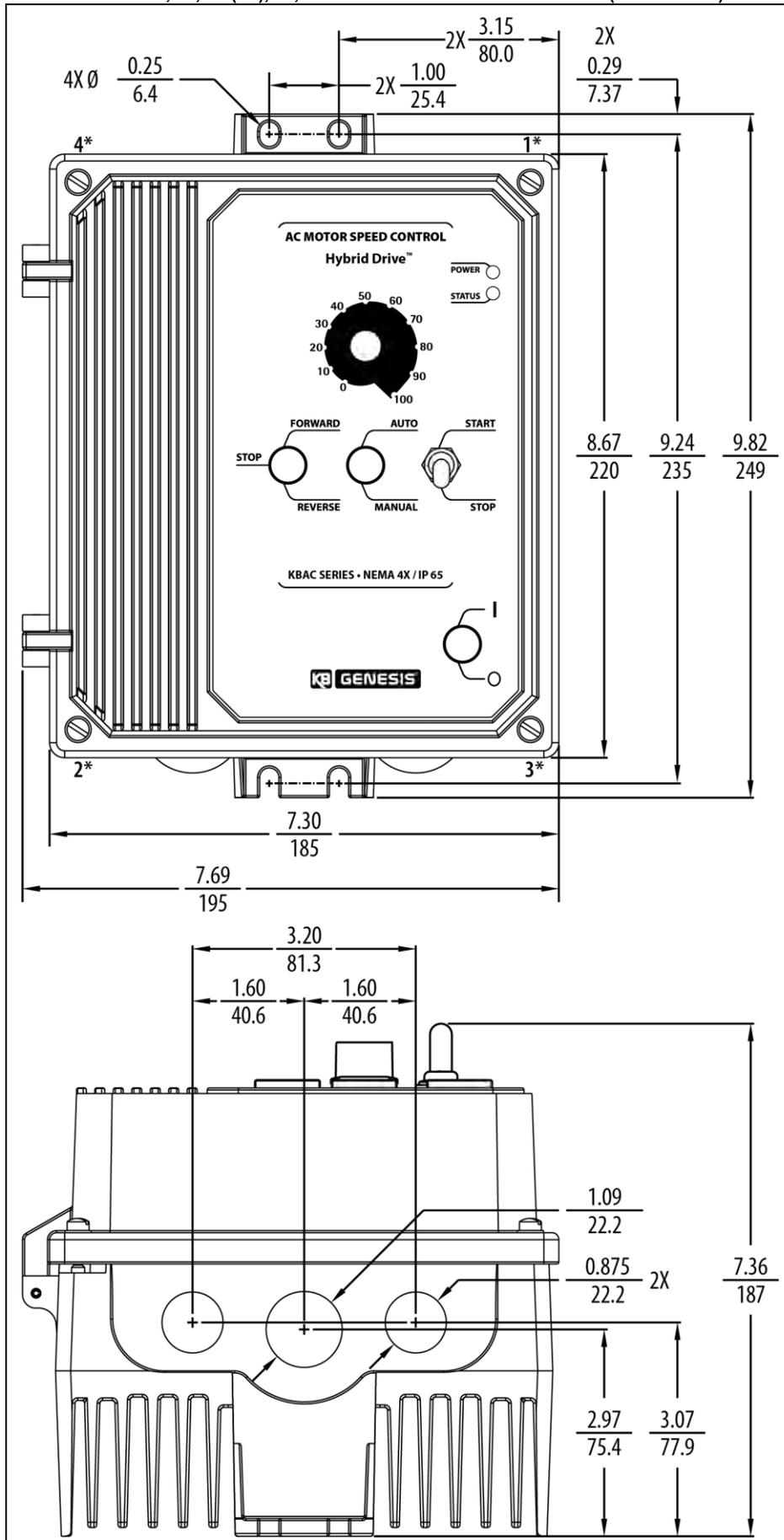
\*Tighten these screws, in the sequence shown, to 12 in-lbs (14 kg-cm).
