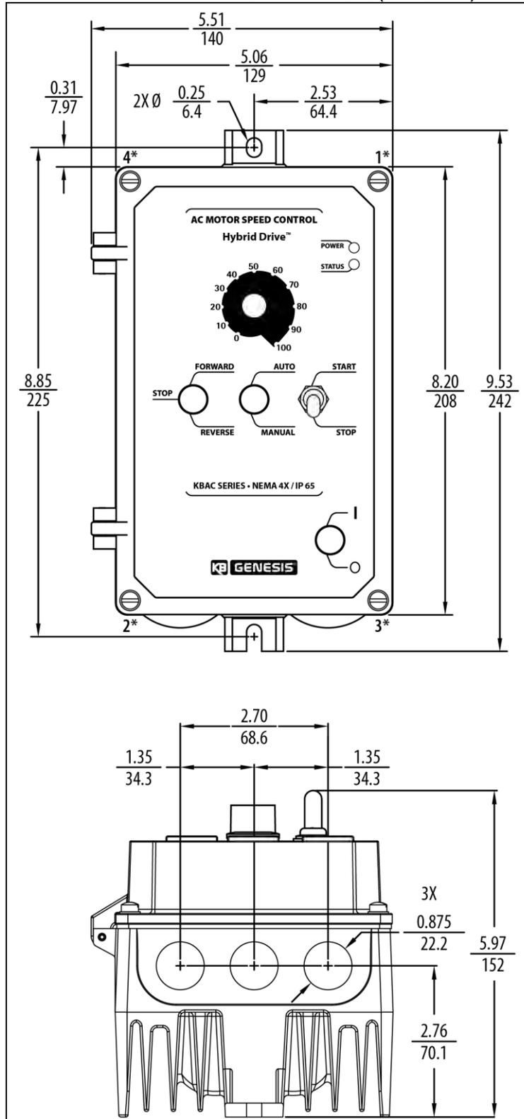
\*Tighten these screws, in the sequence shown, to 12 in-lbs (14 kg-cm).
