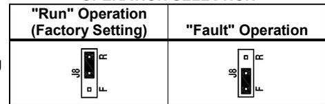
For Run/Fault Relay output contacts, see Section 7.9 on page 18. The Run/Fault Relay contact status for various drive operating conditions is shown in Table 5 on page 18.
