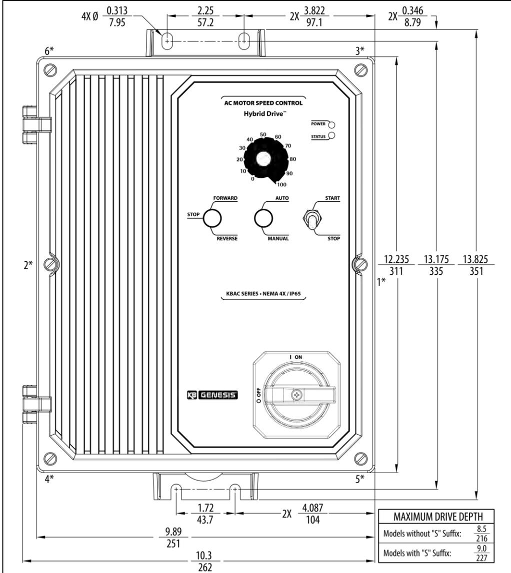
\*Tighten these screws, in the sequence shown, to 12 in-lbs (14 kg-cm).
