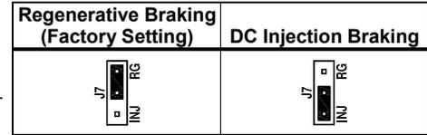
When the Injection Brake Mode is selected, the DECEL Trimpot is used to set the amount of time the DC current is applied to the motor.
