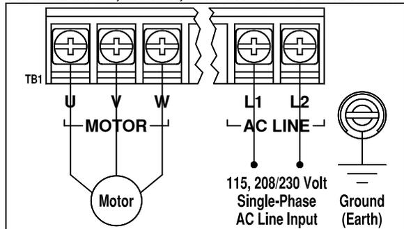
**KBAC-29:** Designed to accept 1-phase (Terminals L1, L2) or 3-phase (Terminals L1, L2, L3) AC Line input. Rated for 208/230 Volt AC Line input only. See Figure 12.
